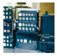
DMS-01 massspectrometric sensor The DMS-01 mass-spectrometric sensor analyses the SSC's own external atmosphere (gas environment) to study the impact of space factors on the quality of scientific and technical experiment and the satellite's aerodynamics.
